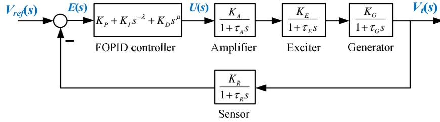
Fig.2. Block diagram of an AVR system with a FOPID controller
