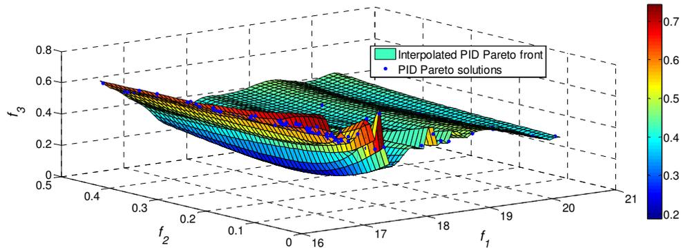
Fig.9. 3D Pareto front of three objectives  $f_1, f_2, f_3$  for MOEO-PID controller
