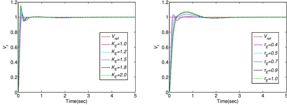
Fig.15. Terminal voltage step response for AVR system with MOEO-FOPID controller under variation of  $K_E$  (left) and  $\tau_E$  (right)
