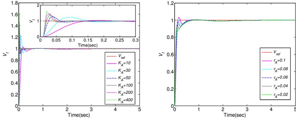
Fig. 17. The terminal voltage step response for AVR system with MOEO-FOPID controller under variation of  $K_A$  (left) and  $\tau_A$  (right)
