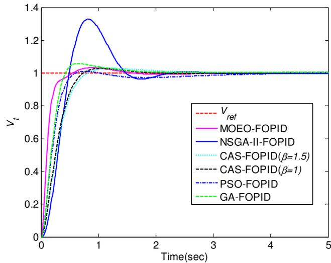
Fig.12. Comparison of terminal voltage step response when  $K_G$  changes to 0.8 from 1 and  $\tau_G$  changes to 1.6 from 1
