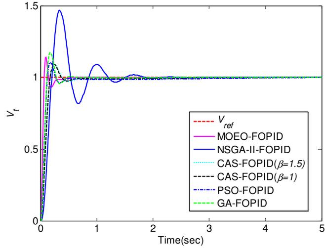
Fig. 16. Terminal voltage step response when  $K_A$  changes to 20 from 10 and  $\tau_E$  changes to 0.07 from 0.1
