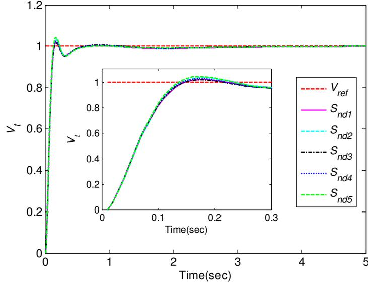
Fig.7. Terminal voltage step response of AVR with representative MOEO-FOPID solutions as reported in Table 3
