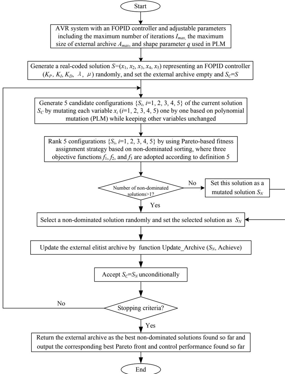
Fig.3 The flowchart of MOEO-based FOPID controller design algorithm
