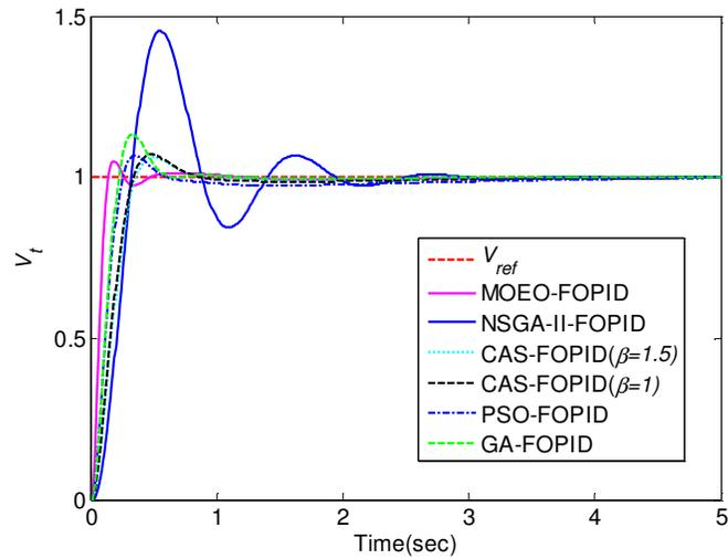
Fig.14. Terminal voltage step response when  $K_E$  changes to 1.2 from 1 and  $\tau_E$  changes to 0.5 from actual value 0.4
