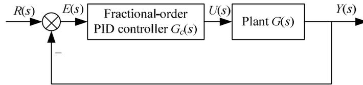
Fig.1. Block diagram of a control system with a FOPID controller
