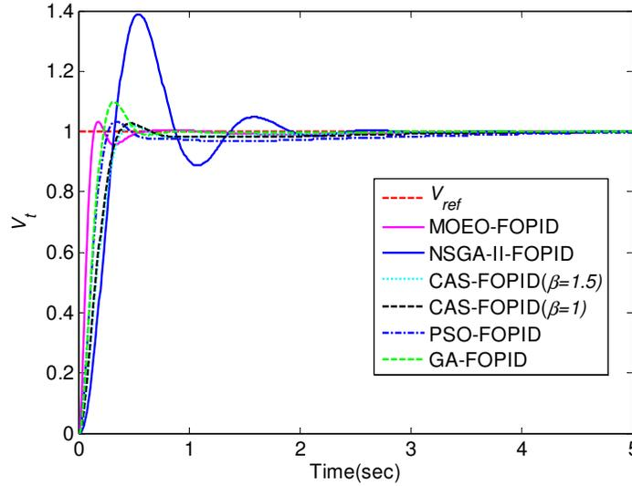
Fig.8. Terminal voltage step response of AVR with MOEO-FOPID, NSGA-II-FOPID and reported competitive single-objective evolutionary algorithms-based FOPID controllers
