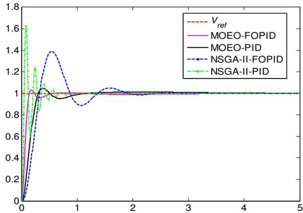
Fig.11. Terminal voltage step response of AVR with MOEO-based with NSGA-II-based FOPID and PID controllers
