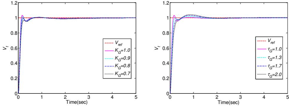
Fig.13. The terminal voltage step response for AVR system with MOEO-FOPID controller under variation of  $K_G$  (left) and  $\tau_G$  (right)
