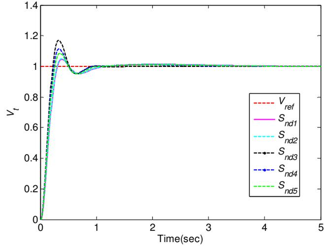
Fig.10. Terminal voltage step response of AVR with representative MOEO-PID solutions as reported in Table 6
